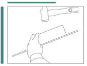
4. Use a tapping block to avoid damaging the strips when fixing them into place.
