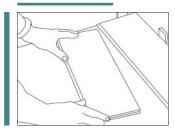
3. Use the offcut of the first row to start the second, ensuring that the offcut is at least twice the width of the strip itself for aesthetic reasons. Immediately remove traces of glue with a slightly damp duster or sponge.
