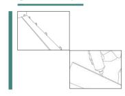
2• Begin laying from a corner. Position the strips with the tongue side against the wall, and carefully glue the top edges of the tongues along their entire length using an aqueous vinyl glue such as Presto BIB. Place wedges around the sides to create an expansion gap.
