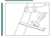
5. Cut the last row of strips to the required width, allowing for an expansion gap. Fix them into place flat with a metal pull bar. 24 hours after laying the floor, remove the wedges and cover the expansion joints using suitable fittings such as skirting boards, radiator rings and threshold strips.
